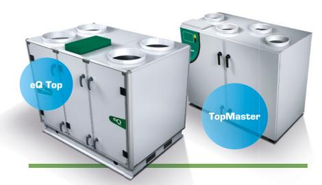
The eQ Top is a compact air handling unit, manufactured in two sizes with an air flow range up to 1,6 m<sup>3</sup>/s. The eQ Top is a flexible air handling unit, which is easy to install and commission. The unit is supplied with direct-driven supply and extract air fans, supply and extract air filters and a rotary heat exchanger. There is a wide range of accessories for the eQ Top for in-duct air processing. This range includes everything necessary such as dampers, coils, silencers etc.
