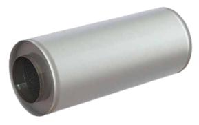
The silencer is a straight circular duct silencer with 50 mm mineral wool filling. Duct connections have rubber seals. The silencer consists of a perforated sheet metal pipe surrounded by a galvanized sheet steel mantle and end pieces sandwiching mineral wool covered with nonwoven fabric to prevent fiber migration.
