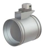
Duct mounted damper in leakage class 3 (CEN 3). The damper is made of galvanized sheet steel and has a spring return on/off actuator. The actuator has to be connected to a terminal block in the electrical cabinet.
