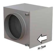
Cold water coil containing copper tubes and aluminum fins. The coil is built-in to a galvanized sheet steel casing. The casing has a removable hatch for cleaning and duct connections with rubber ring seals. The cooler has to be installed horizontally and the distance to nearest bend has to be at least 600 mm. The cooler is only available in a left-hand version.
