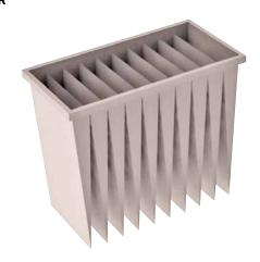
Green Flo bag filter made of PLA for low pressure drop. Filter class F7 on both supply and extract air. The filters are pressed against the sealing strip in the casing.
