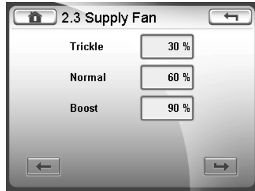
Make the appropriate settings for the supply fan and press the confirm button.
