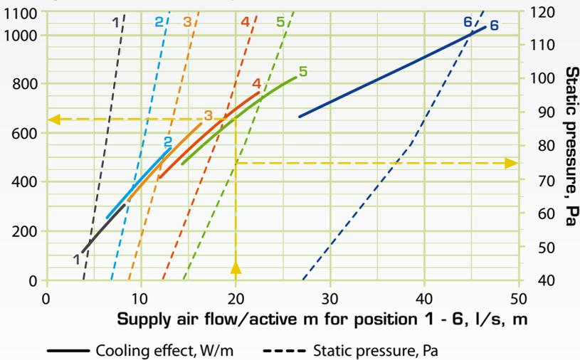
The diagram shows the approximate cooling effect  $P_{tot}$  in W with water flow  $q_w = 0.1$  l/s, temperature difference between room air and supply air  $\Delta t = 8^\circ\text{C}$ , pressure drop 70 Pa on the air side and max. sound pressure level  $L_{A10} = 30$  dB(A).
