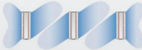
When increased air flow is required, the flow pattern can be adapted to maintain optimal comfort in the room!
