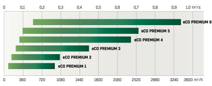
eCO PREMIUM<sup>™</sup> is available in 6 sizes providing from 0,2–0,9 m³/s of air flow. A range appropriate for a wide range of applications and building sizes.
