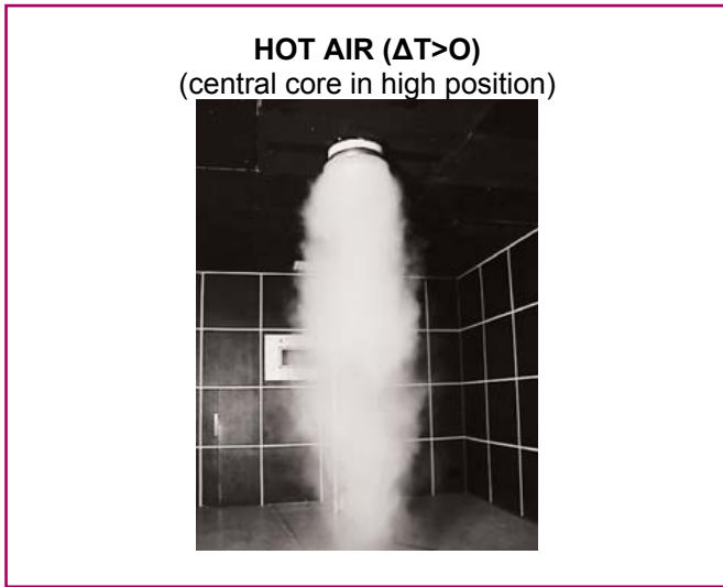
Photographs of DGV diffuser tests in the R&D Laboratory of KOOLAIR S.A.
