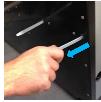
Picture 3: Finally remove the strap from the the dehumidifier.
